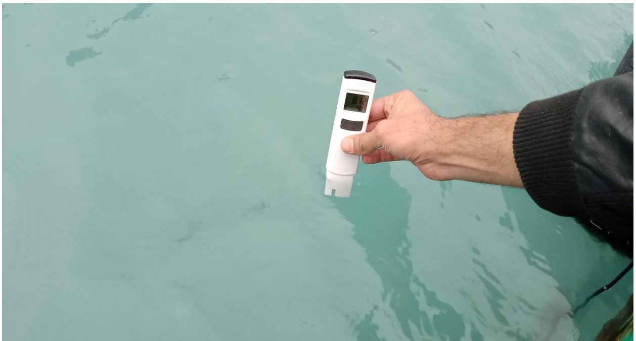
Photograph 36: Testing of Lake Water with Portable PH Meter
